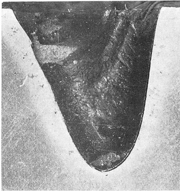
Fig. 4 Photograph of a cross section of a crater after polishing, X6 magnification
